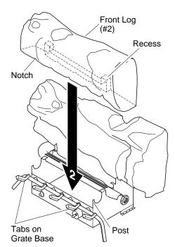
Figure 36 - Installing Front Log
